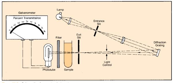
Figure 23.5 Schematic of a spectrophotometer
