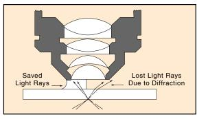
Figure 1.8 Immersion oil, having the same refractive index as glass, prevents light loss due to diffraction.
