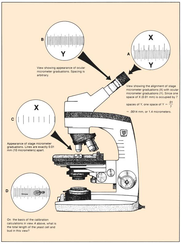
Figure 5.4 Calibration of ocular micrometer
