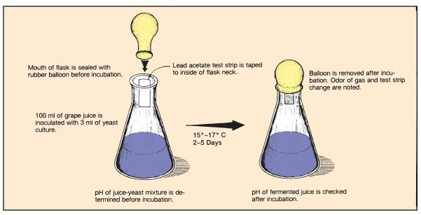
Figure 72.1 Alcohol fermentation setup
