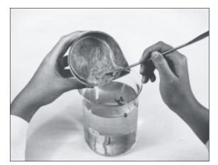
Figure 20.3 Dehydrated medium is dissolved in a measured amount of distilled water.
