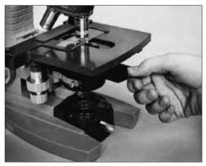
Figure 3.9 The annular stop on this American Optical microscope has the annular stop located on a slideway. When pushed in, the annular stop is in position.
