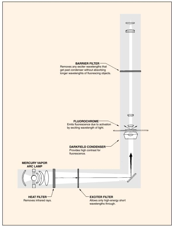
Figure 4.2 The light pathway of a fluorescence microscope
