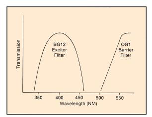
Figure 4.3 Spectral transmissions of BG12 and OG1 filters
