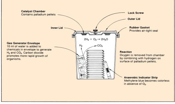
Figure 22.2 The GasPak anaerobic jar
