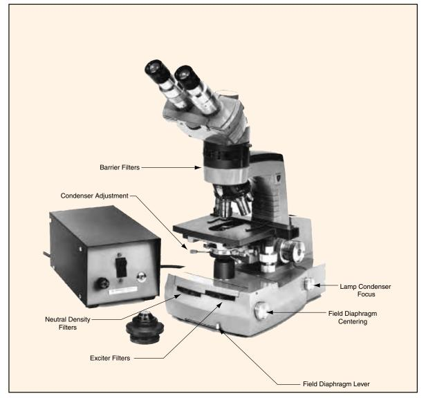
Figure 4.4 An American Optical fluorescence microscope
