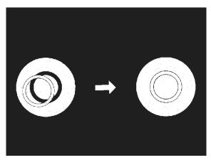
Figure 3.4 The image on the right illustrates the appearance of the rings when perfect alignment of phase ring and annulus diaphragm has been achieved.
