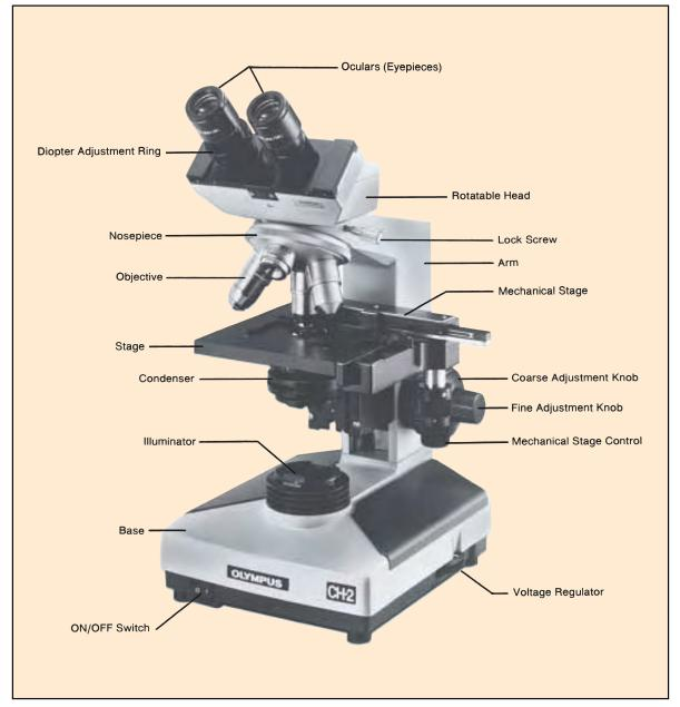
Figure 1.2 The compound microscope
